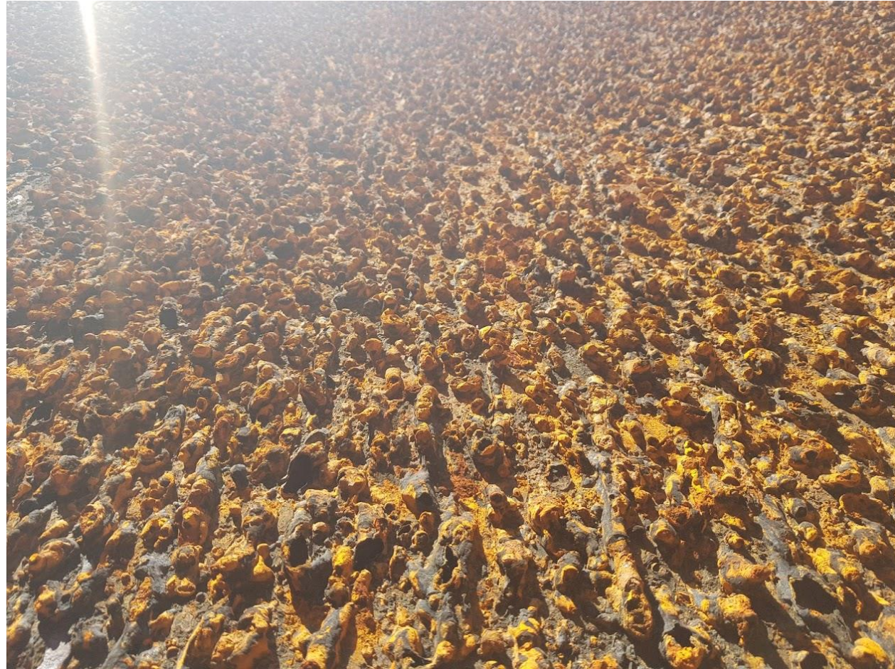
Example of a surface that cannot be measured with the RoNik UT drones
